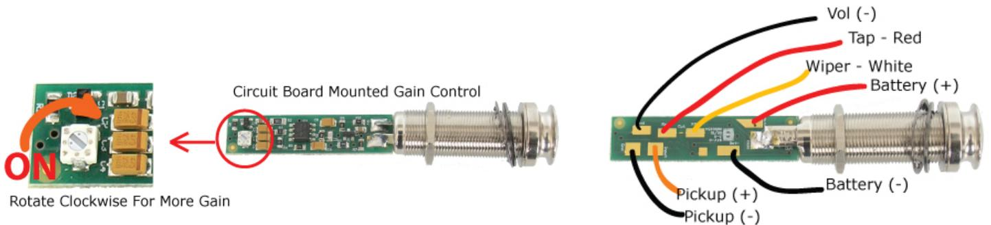
**Installing the Pickup**
